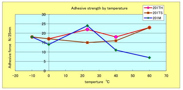
Measure at room temperature after leaving the SUS laminated test specimen for 2 hours under a prescribed temperature atmosphere. (Test conditions are the same as 1)
