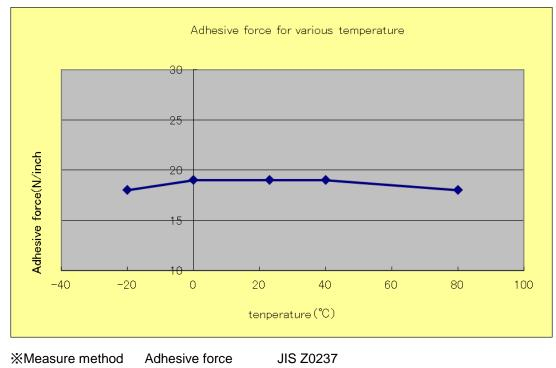
Adhesive force PET#25 backing, peeling speed 300mm/min, 180° angle.
